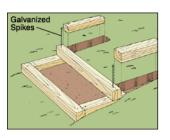
Excavate between the sides, as before. Continue up the hillside in this fashion. When installing the top step, cut the side timbers 6" shorter than the ones on the lower steps - these timbers do not need the extra length since no stairs will rest on them.
